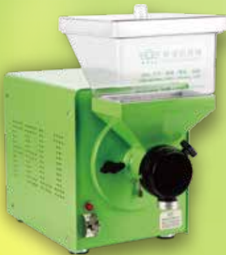
NBM-100 Nut Butter Grinder 46x25x44cm / 30kg 1.25HP / 1800RPM
